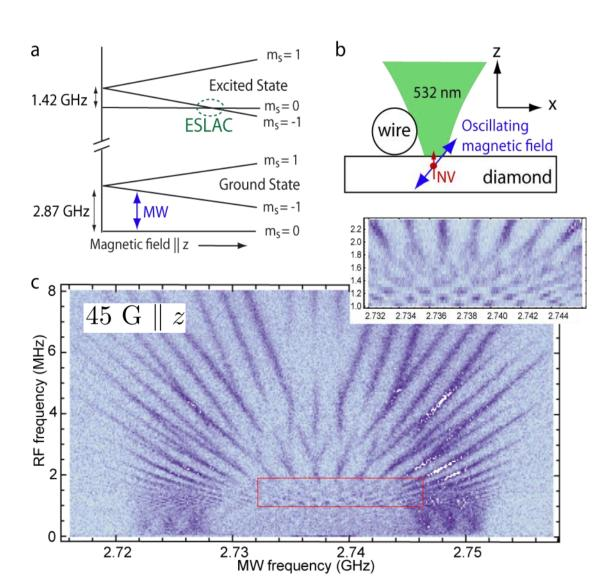
Experiments by Childress and McIntyre [4]: Simultaneous excitation by weak MWs to drive electronic spin transitions and strong radio-frequency excitation to drive nuclear spin resonance:
