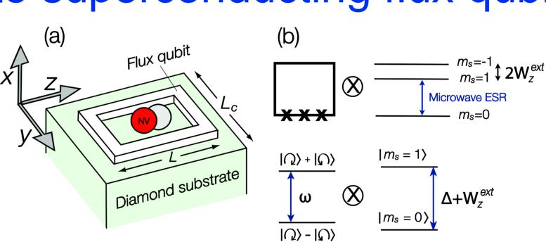
A new hybrid qubit is proposed, a flux qubit coupled to an ensemble of NV centers in diamond.
