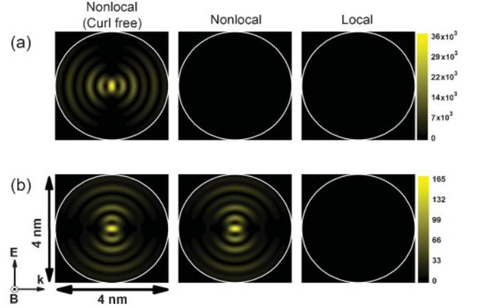
FIG. 2. (Color online) Field distributions in the three different models, for TM-polarized light normally incident on a cylinder of radius  $a = 2$  nm. (a) Normalized displacement field  $|D|^2/|D_{\text{in}}|^2$  at the frequency  $\omega = 0.6503\omega_p$  (P1 in Fig. 1).  $D_{\text{in}} = \varepsilon_0 E_{\text{in}}$  and  $E_{\text{in}}$  is the incident electric field. (b) Analogous plots of  $|E|^2/|E_{\text{in}}|^2$  for  $\omega = 1.1963\omega_p$  (P2 in Fig. 1).
