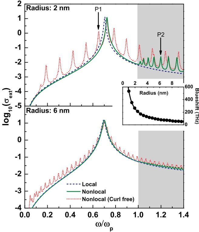
FIG. 1. (Color online) Extinction cross sections  $\sigma_{\text{ext}}$  as a function of frequency for TM-polarized light normally incident on a metallic cylinder in vacuum. Parameters for Au as in Ref. 14:  $\hbar\omega_p = 8.812$  eV,  $\hbar\gamma = 0.0752$  eV, and  $v_F = 1.39 \times 10^6$  m/s. Inset: Frequency shift of the maximum  $\sigma_{\text{ext}}(\omega)$  for nonlocal against local response, as a function of radius.
